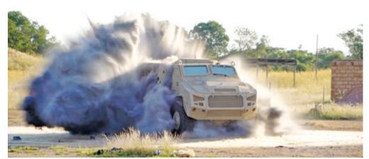
Paramount Group, the global technology and aerospace business, has announced that the Mbombe 4x4, the newest addition to its advanced Armoured Personnel Carrier (APC) family of vehicles, has received final certification for the independently verified blast tests which exceeded the criteria for NATO STANAG 4569 – one of the highest levels of protection that can be achieved by an armoured vehicle in its class.
